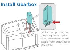
Power off. Open the top lid Install one gearbox according to the sample type. Close the top lid.
