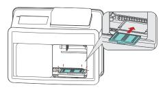
Open the door. Install the corresponding heating block.
