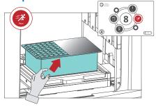
Remove the aluminum foil carefully. Place the extraction kit with cropped corner facing outwards. Tap **Run** icon. **Note:** Aluminum foil should be fully remove while operate with CH16 Gearbox
