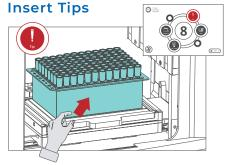
Tap **Tip** icon and place a tip box on the heating block.
